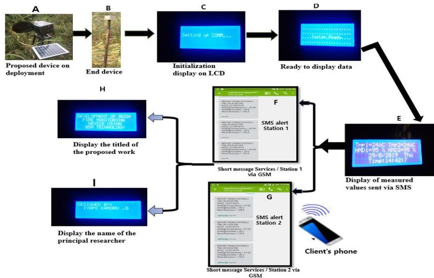
Fig.10. LCD screen showing display result during Hardware deployment
