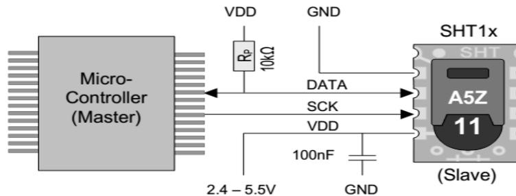
**Fig.4.** Microcontroller interface to the STH11 sensor.
