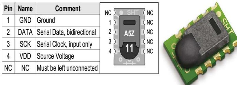
**Fig.5.** The SHT11 temperature humidity sensor interface Specifications
