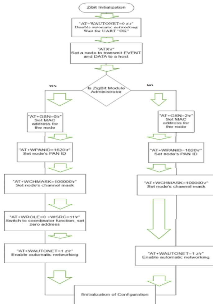
Fig.9. Flowchart for the ZigBee Module Configuration
