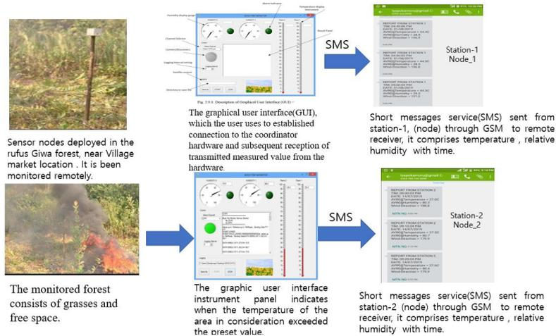
Fig.12. show Graphic user Interphase(GUI) and data received via SMS during hardware deployment
