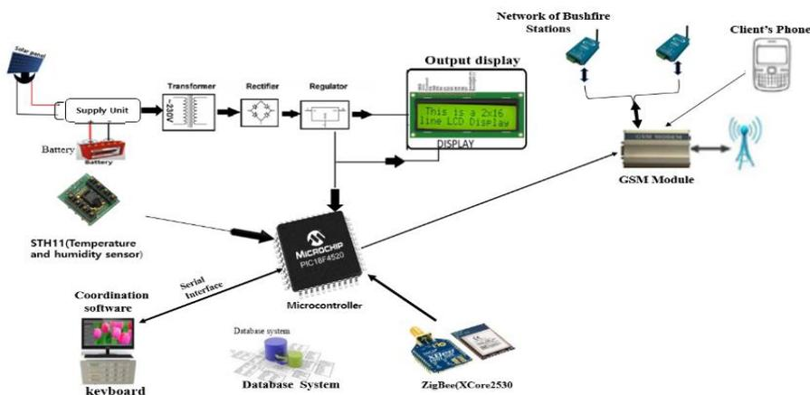
Fig.1. Block diagram of the proposed bushfire monitoring system.
